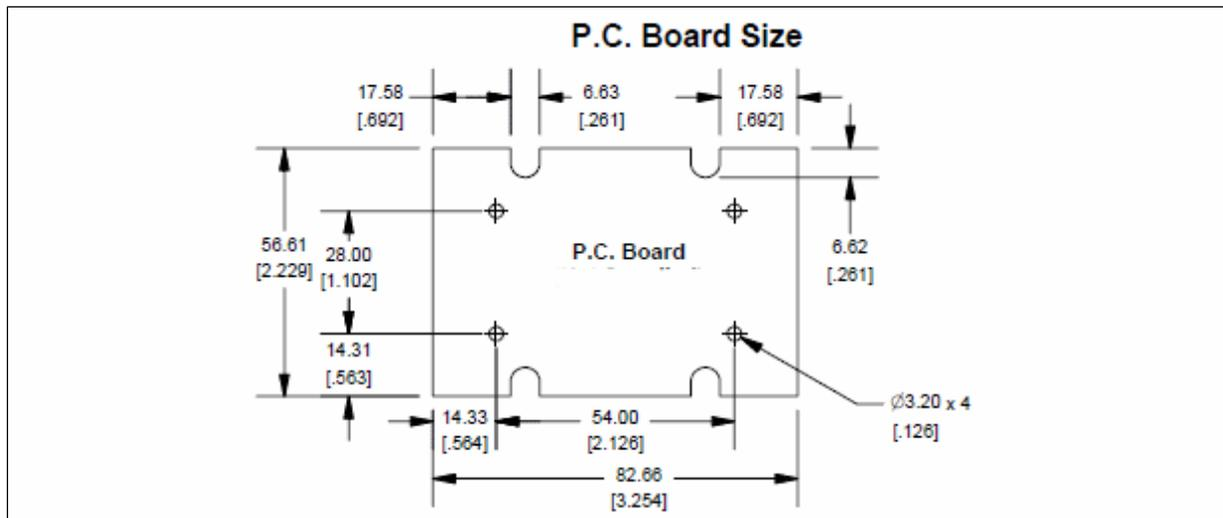
Fig. 5: Module PCB dimension details in mm and [inches]
