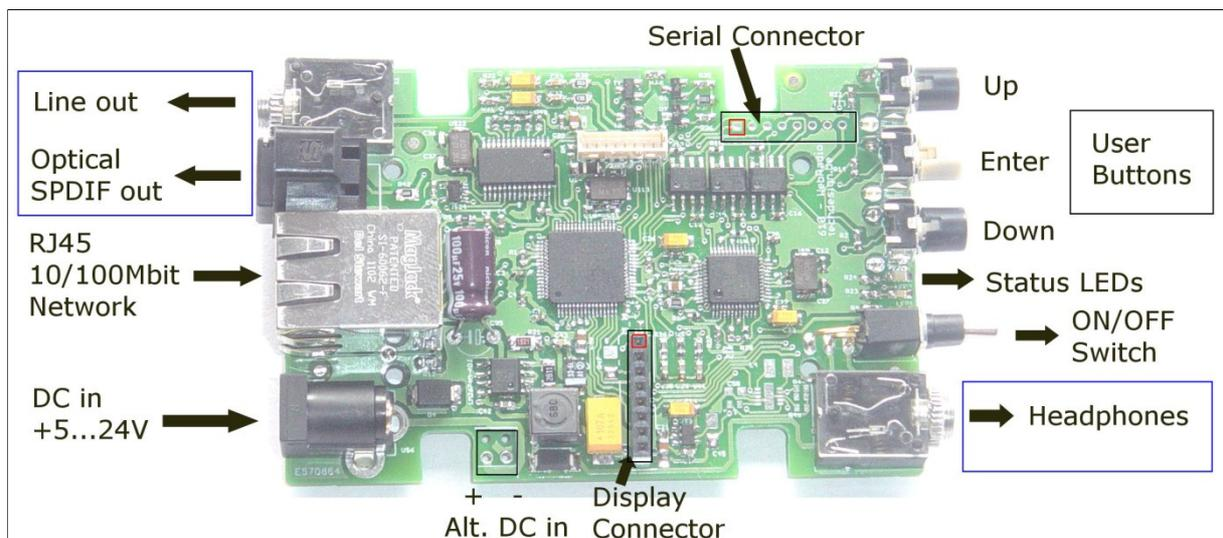
Fig. 1: WebRadio Module WR1-AD: Connection overview.
